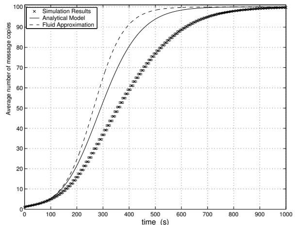
Fig. 8. Average number of message copies in the network versus time,  $N = 100$ , Random Waypoint Mobility model,  $v = 4$  m/s,  $R = 50$  m .
