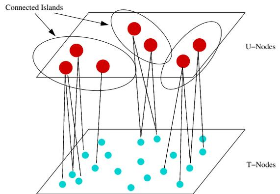
Fig. 1. The two-tier SOCS network architecture.
