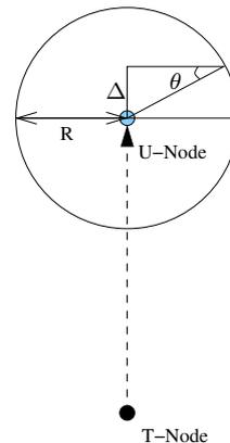
Fig. 5. Geometrical representation of the meeting process.  $\theta$  defines the angle between the velocity vectors of the two devices and  $\Delta$  the progress in the radial direction.
