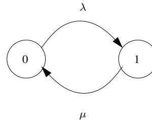
Fig. 2. Model of the process  $X(\cdot)$ , sampled by the sensor node, as a two-states Markov chain.
