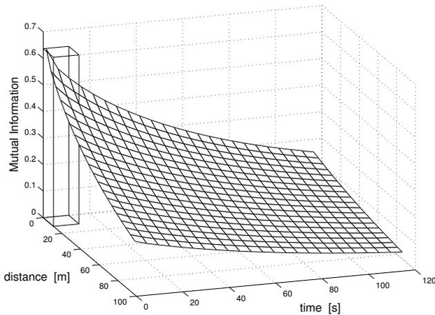
Fig. 3. Mutual information function versus time and space lags,  $\lambda = 0.0033$ ,  $\mu = 0.0017$ ,  $\gamma = 0.0050$  and  $\varepsilon = 0.2$ .
