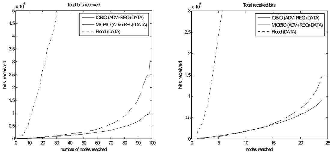
Figure 3. The total bits received by the nodes when the  $N^{\text{th}}$  node is reached using the RPGMMDC. In the left picture the results are shown when 100% of the nodes were in the same UC, while the picture on the right shows when only 25% belonged to the examined UC
