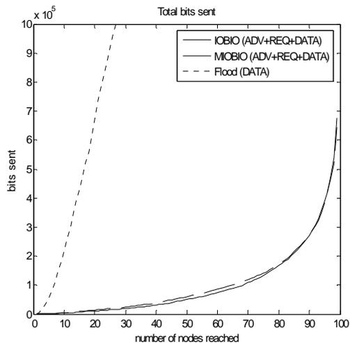
Figure 1. The amount of data that is needed to reach the  $N^{\text{th}}$  node
