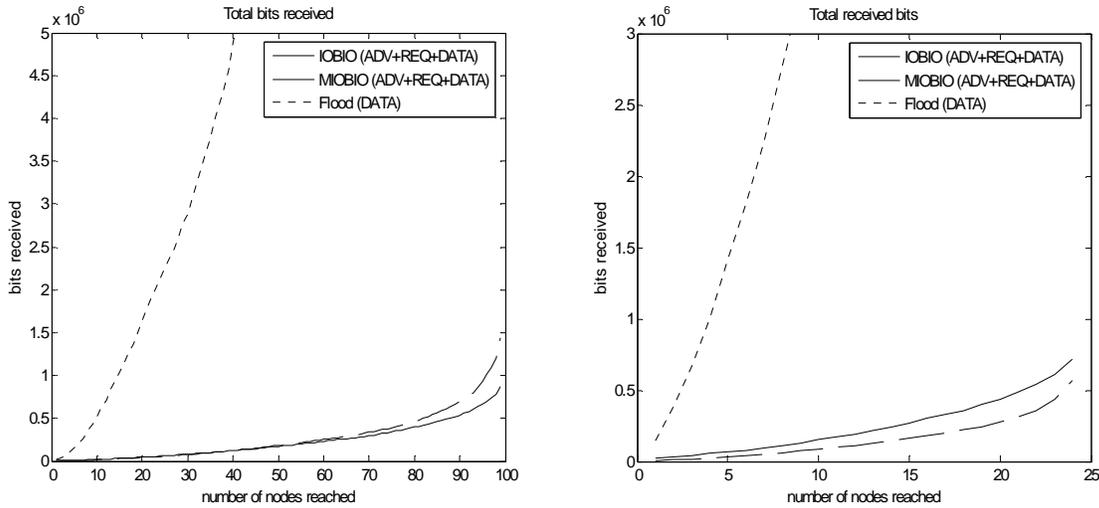
Figure 2. The total bits received by the nodes when the  $N^{\text{th}}$  node is reached using CSMM. In the left picture the results are shown when 100% of the nodes were in the same UC, while the picture on the right shows when only 25% belonged to the examined UC
